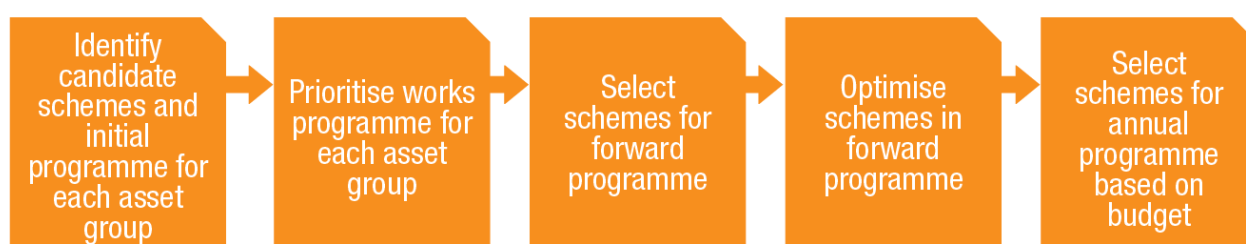
Figure 8.3 – Developing a Programme of Works, HMEP Highway Infrastructure Asset Management Guidance, Figure 6, Page 53
